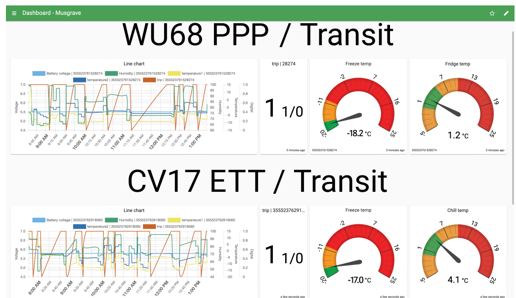
Figure 3. Developed dashboard shows environmental parameters in real time.
