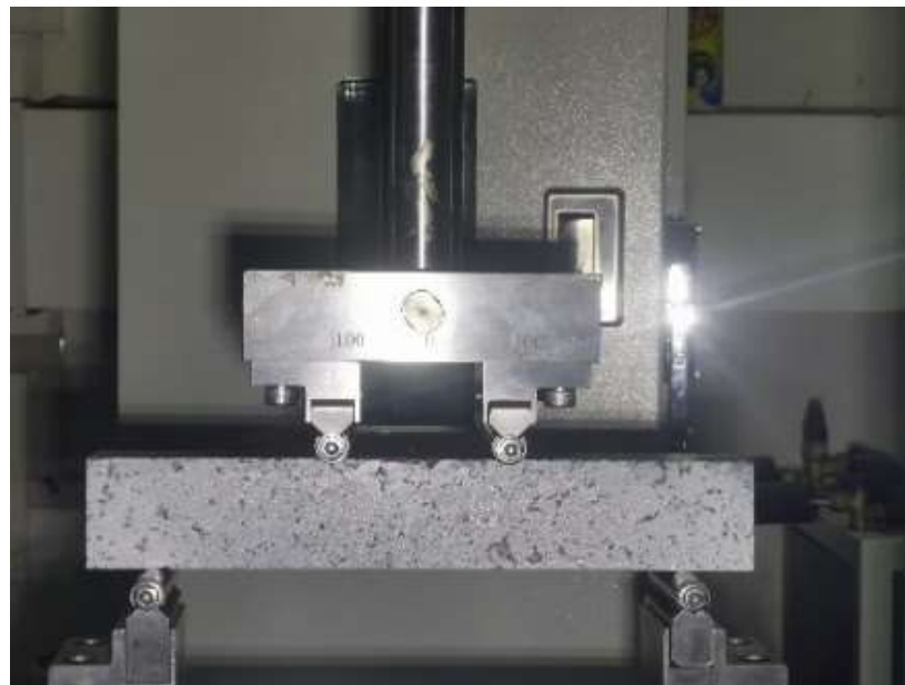
Figure 2. Four-point bending loading layout.
