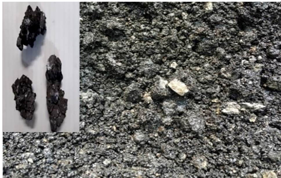
Figure 6. Illustration of surface milling at low temperature.
