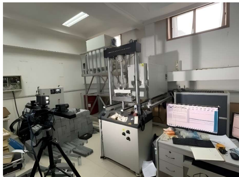
Figure 3. Fatigue loading and DSCM acquisition site.
