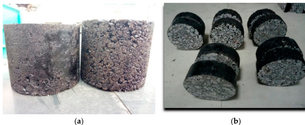
Figure 3. The preparation process of asphalt mixture specimen: (a) After rotary compaction; (b) After cutting.
