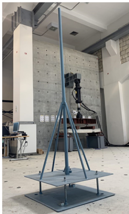
Figure 4. Impact test drop-weight frame.
