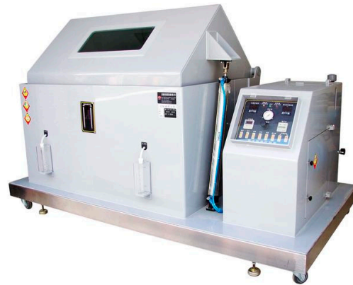
Figure 1. Automatic machine for cyclic exposure to salt spray conditions.
