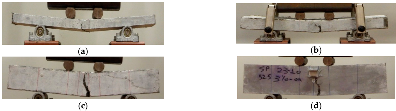
Figure 4. Characteristic failures of selected typical prisms for (a) 25 mm, (b) 50 mm, (c) 75 mm and (d) 100 mm depths.
