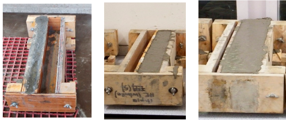
Figure 1. Preparation of prisms with different depths.
