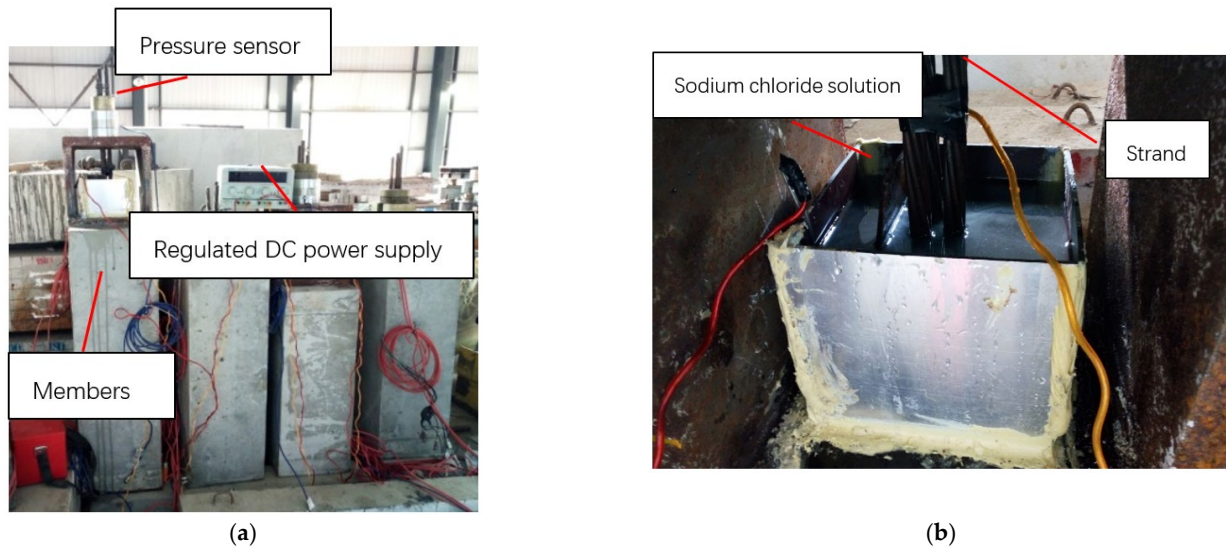
Figure 2. Corrosion position of test members: (a) corrosion process of specimen; (b) detailed structure of corrosion groove.
