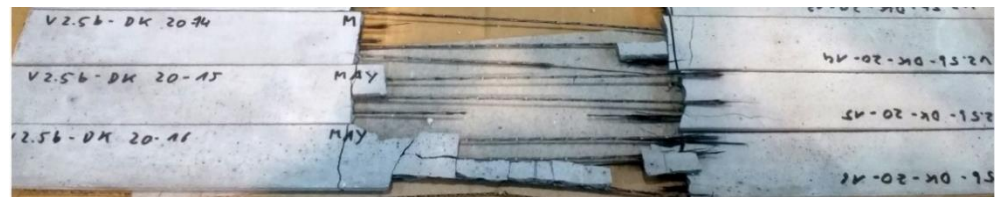
Figure 15. Tensile test specimen of concrete embedded rovings after failure.
