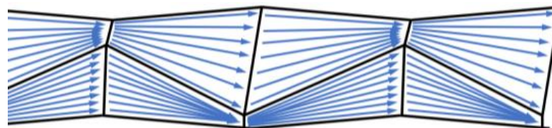
Figure 3. Schematic filament orientation of tetrahedral profiled rovings.
