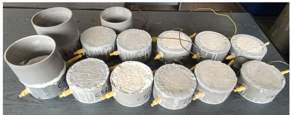
Figure 1. Specimens of both types of concrete prepared for testing during curing.
