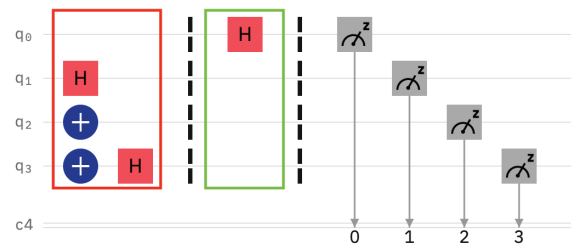
Figure 6. Four positional sentinels are set to all possible values. The experiment shows the option where the intruder is lucky on only one qubit, namely q_2 .
