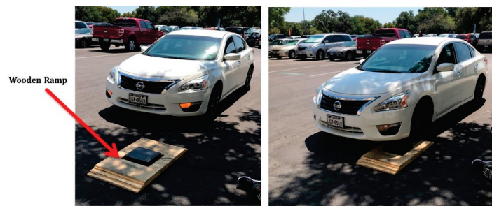
Figure 13. Road testing of the HiSEC module with the TTN ethernet gateway placed 30 m from the ramp.
