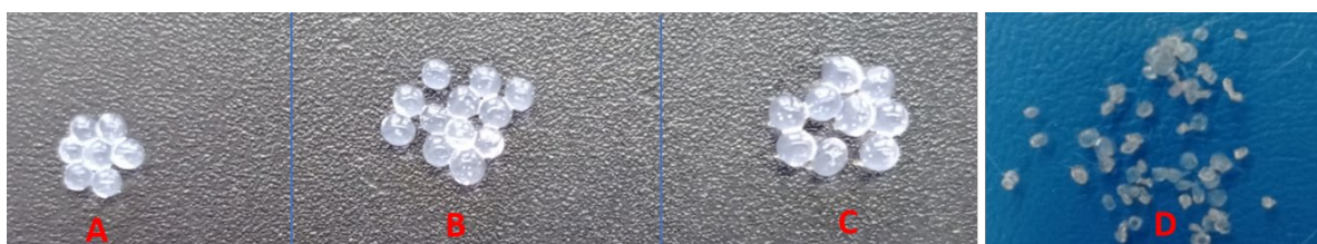
Figure 2. The appearance of beads: Alg (A), Alg/BC (B), Alg-PUL/BC (C), and dehydrated (D) beads.
