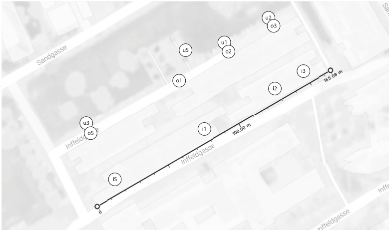
Figure 1. Deployment map for our experiments indoor (i), outdoor (o), and underground (u). The sender node for each scenario is indicated with iS, oS, and uS, respectively.
