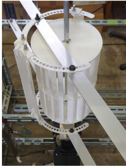
Figure 6. Setting appearance of a cross-flow wind turbine test model with three flow deflectors.
