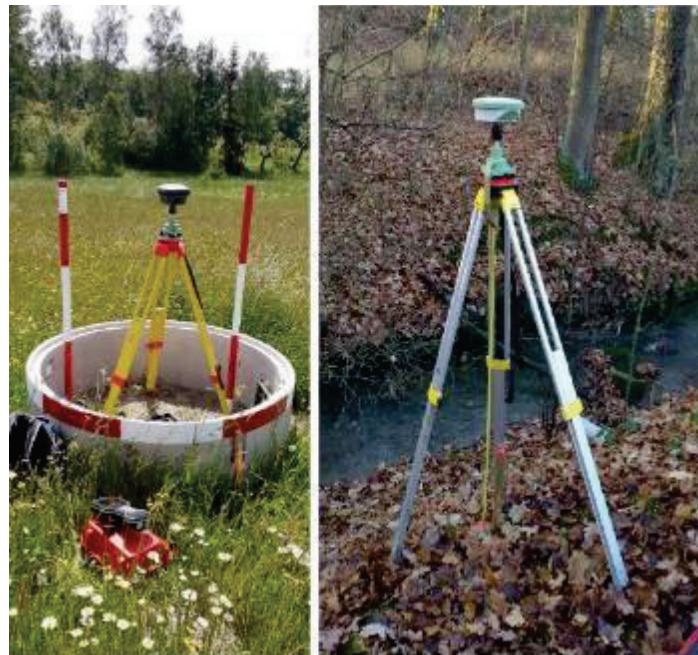
Figure 2. Fast static method; reference station (left); rover (right).
