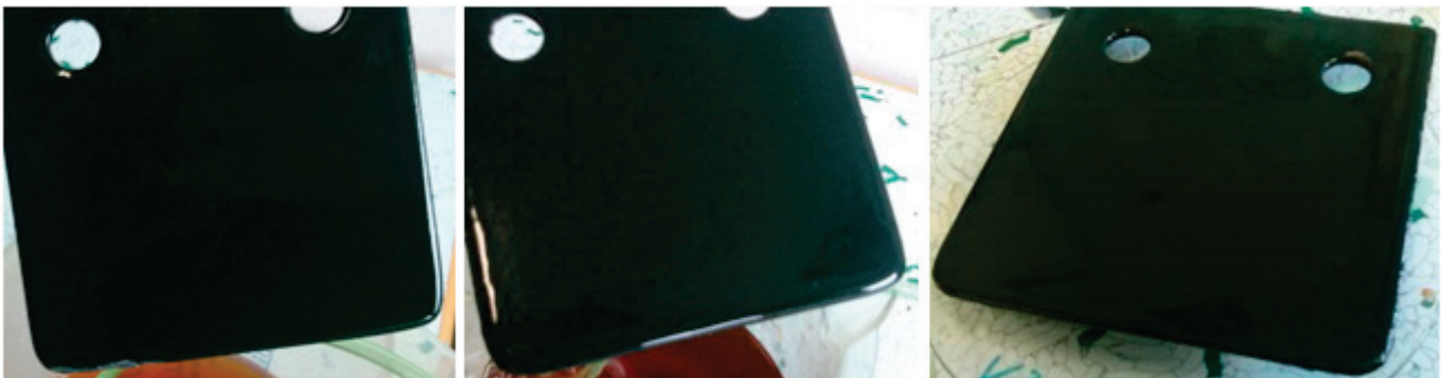
Figure 2. Damage to the edges of samples 1 to 3 (from left to right) after 15 days of leaching.
