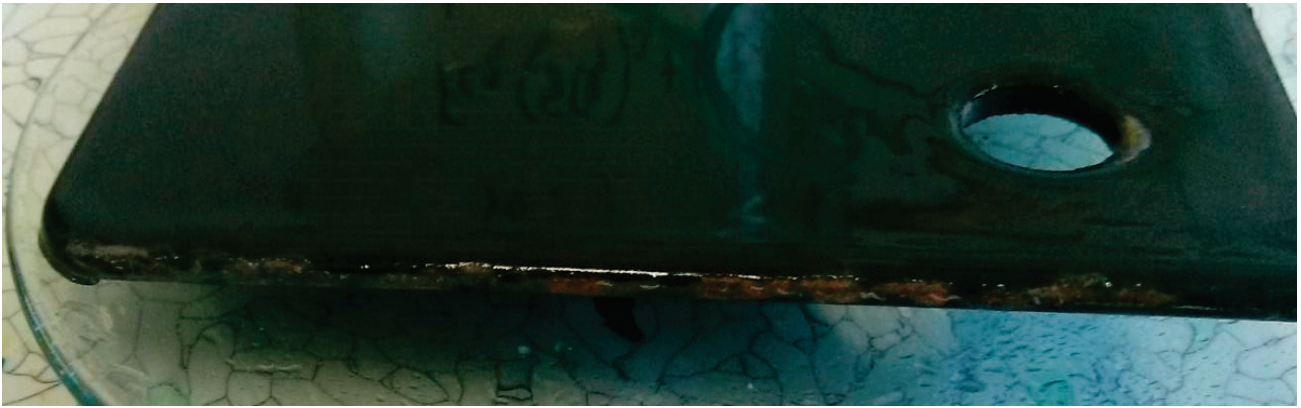
Figure 4. Detail of sample 3's damaged edges after 15 days of leaching.
