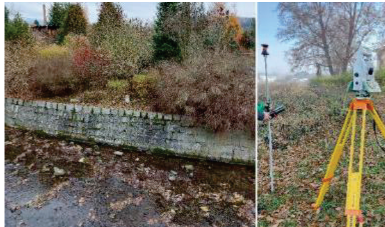
Figure 3. Detailed surveying of the river using a total station.
