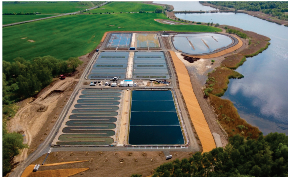
Figure 1. Aerial view of the biotechnological unit of the water treatment plant. Tanks A1, B1, C1 in the left line, A2, B2, C2 in the right line, retention tank D in the upper right.
