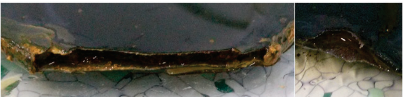
Figure 6. Portals formed by the enamel during the degradation of the base plate.
