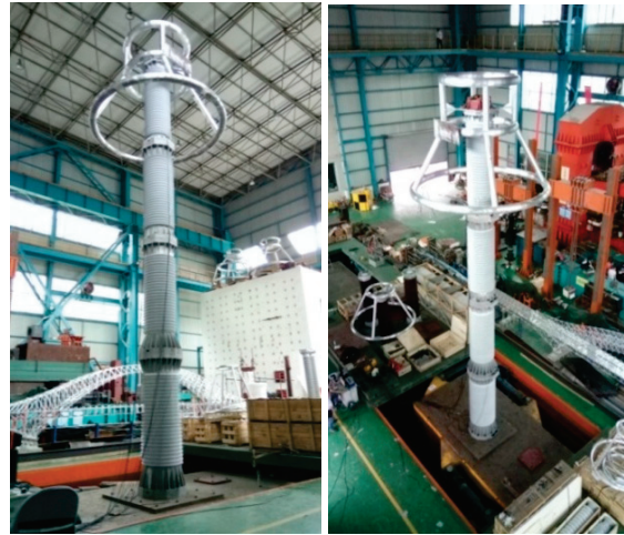
Figure 16. Shaking table test of the 1000 kV surge arrester with GFRP insulators.
