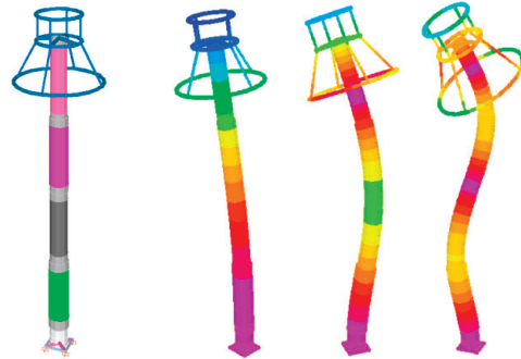
Figure 7. FE model of the 1000 kV surge arrester (left) and the first three mode shapes (right).
