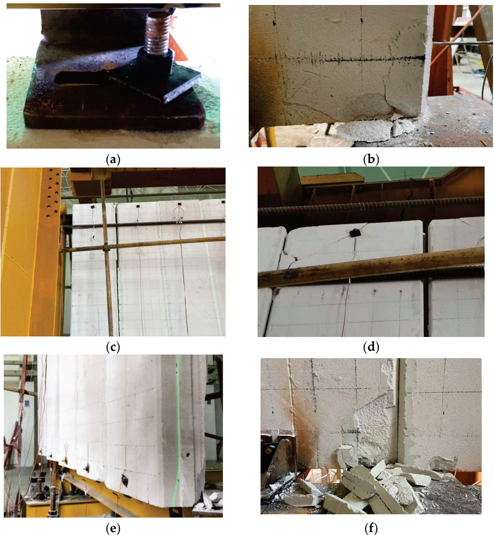
Figure 9. Experimental results of SFW2: (a) upper connector slipped within bolt hole; (b) corner panel was broken; (c) splicing mortar broke and relative movement; (d) cracks appeared at the upper bolt holes; (e) obvious interpanel dislocation; (f) corner of the panel back was broken off.
