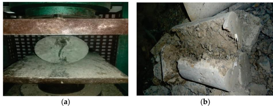
**Figure 7.** (a) The splitting tensile load application on a cylindrical specimen; and (b) the failure of the specimen after the test.
