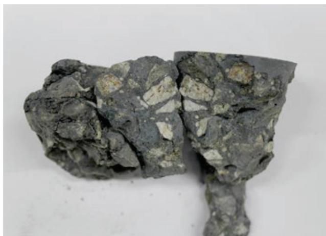
**Figure 1.** Fracture surface showing cracking through aggregate particles in geopolymer concrete.
