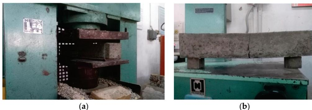
Figure 9. (a) Flexural testing setup for Prismatic specimens of length 500 mm; and (b) the failure of a specimen after the test.
