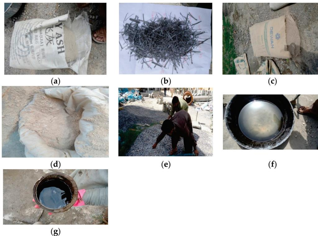
**Figure 1.** The materials used in the present study to produce QRD incorporated FA and SG-based GPC (QFS-GPC) reinforced with steel fibers; (a) fly ash, (b) ground granulated blast furnace slag, (c) steel fibers, (d) quarry rock dust at site, (e) aggregates, (f) alkaline solution, and (g) superplasticizer.
