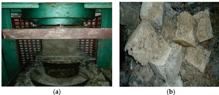
Figure 5. (a) The compressive testing of cubes; and (b) the failure samples.
