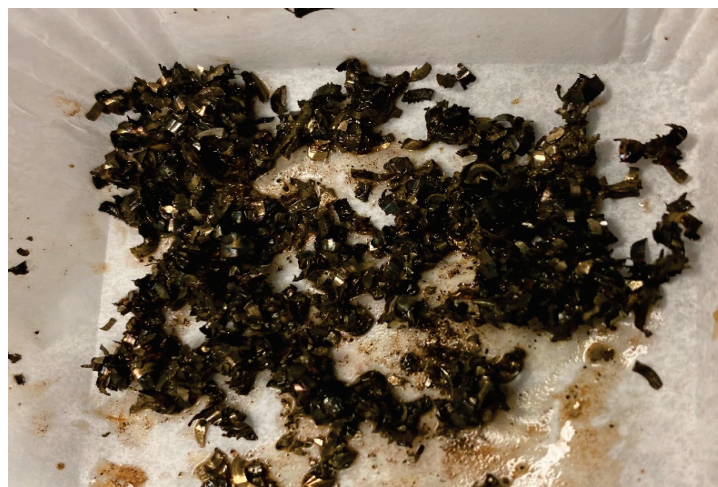
Figure 1. Seymchan meteorite (shavings) post 8 years corrosion reaction at room temperature.
