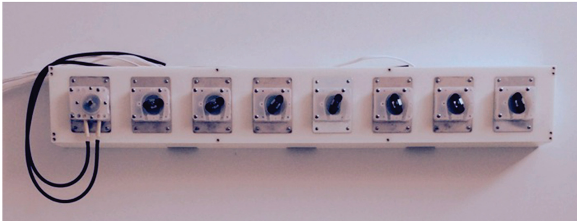
Figure 4. Peristaltic pump array permitting every flask to be connected to the central receiving flask from which every other flask can be reached. The Viton tubing is shown connected only to the left-most pump and the wiring connecting the pump array to the custom programmable electronic control box is visible at the extreme left.
