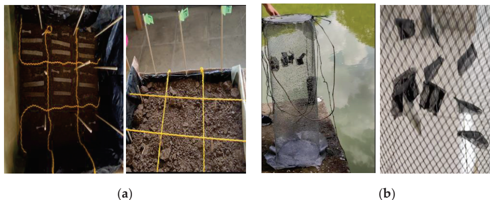
Figure 2. Degradation setup: (a) soil and compost and (b) water.
