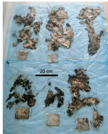
Figure 5. Photographs of samples from prototype 1–6 after 61 weeks of outdoor weathering.
