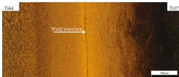
Figure 3. Cross section of the linear friction welding (LFW) joints with Ti64 and Ti17 alloys.
