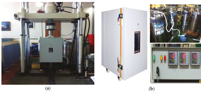
Figure 5. Test equipment: (a) servo hydraulic testing machine; (b) temperature control system.
