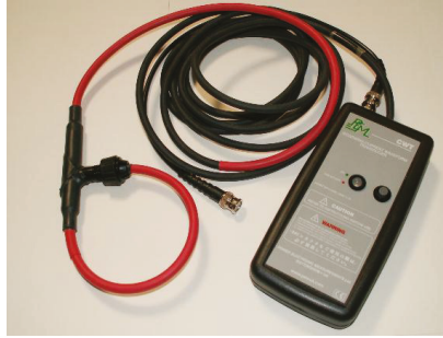
Figure 3. The electrical transducer (Rogowski coil and integrator device) used in the welding tests [14].
