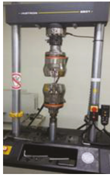
Figure 6. Test equipment (10 tons, Instron 8801).
