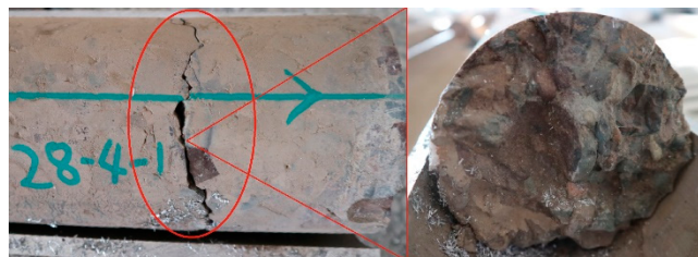
Figure 12. Core cutting-induced fracture in a slant core. Fracture morphology is highly closed and serrated. Fracture surface is fresh with no drilling mud.
