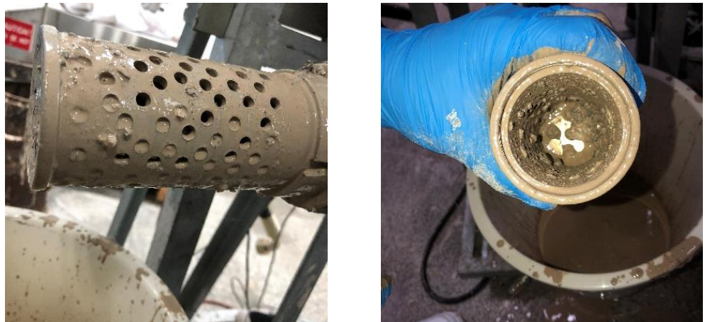
Figure 8. LCMs pass smoothly through the mud screen tool.
