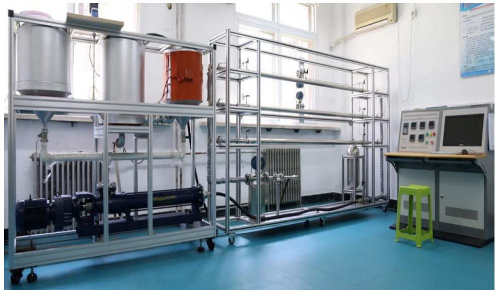
Figure 1. Loop flow drag test system.
