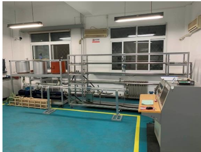
Figure 1. Picture of the loop friction test device.
