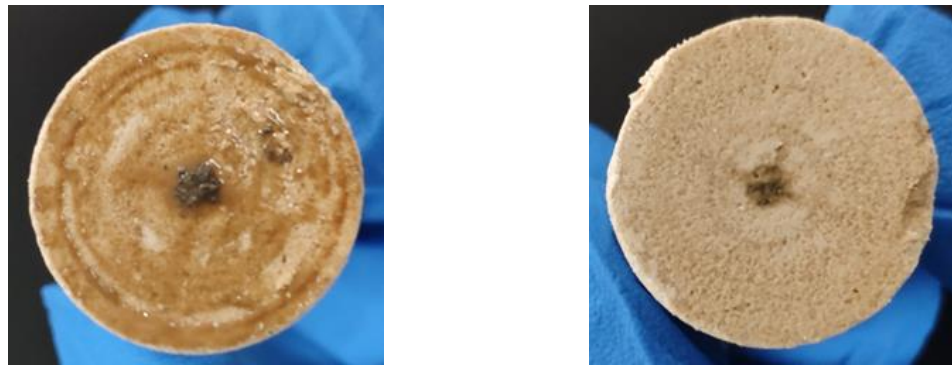
Figure 13. Core inlet (left) and outlet (right) after damage.
