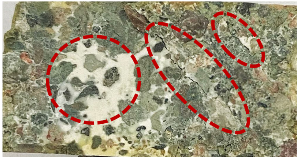
Figure 6. Acid marks and obvious fractures after acidizing.
