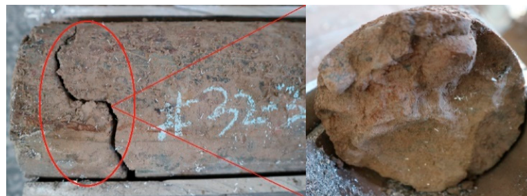
Figure 11. Drilling-induced fracture in slant core with irregular twisted fracture morphology. Fracture surface comprises bypassing gravel with drilling mud attached.
