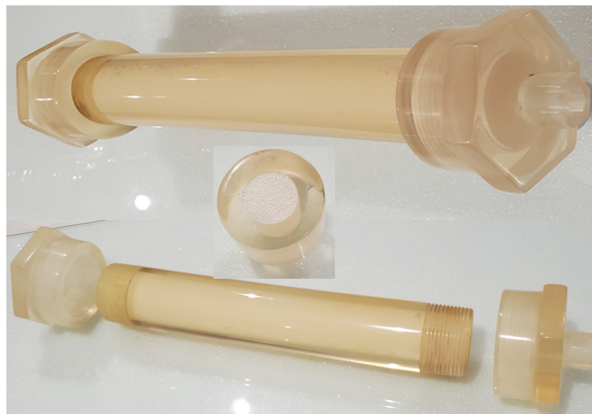
Figure 6. Three-dimensionally printed array core plug and core holder for core flooding tests.
