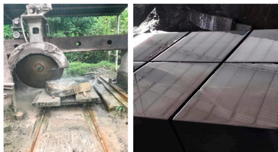
Figure 2. Process of cutting a shale outcrop.
