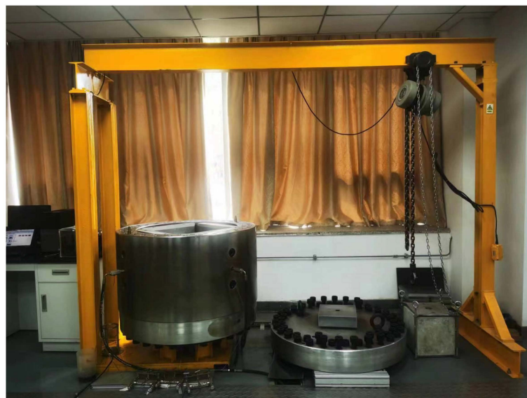
Figure 1. The real tri-axial large-scale hydraulic fracturing initiation and propagation physical simulation system.
