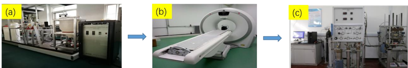
Figure 3. Equipment for acid etching and conductivity test: (a) Rock slab acid etching device, (b) CT scanner, (c) Fracture conductivity test.
