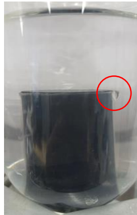
Figure 8. Expulsion of oil from the core during the imbibition process. The red circle marked kerosene that had been released from the shale core.
