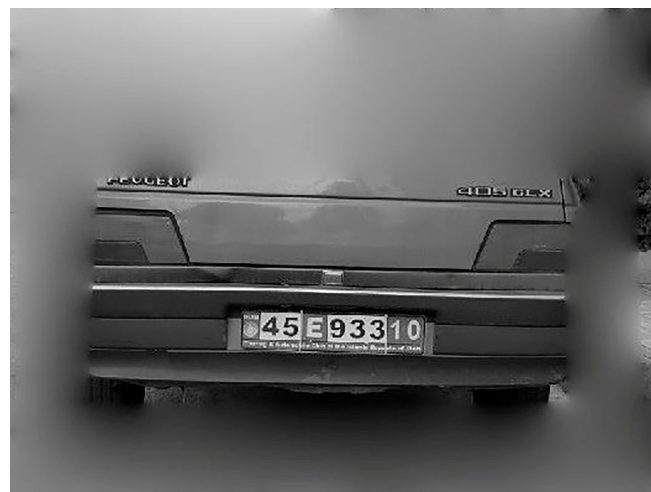
Figure 4. A typical image affected by Blur filter; non-useful areas have been blurred.
