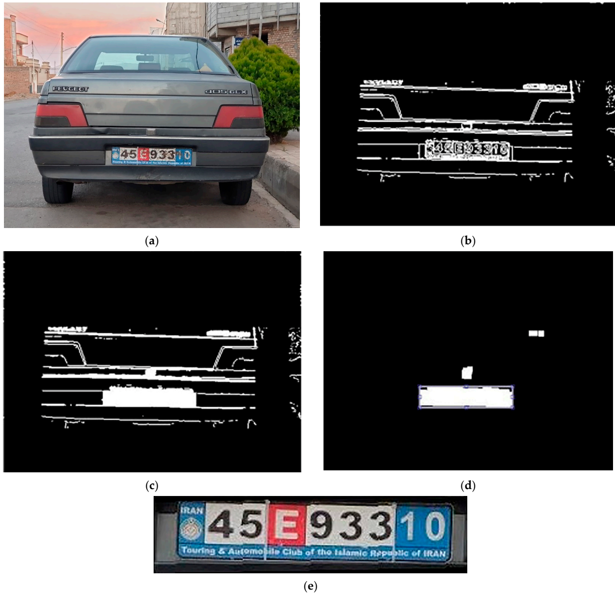
Figure 7. Detecting the license plate frame: (a) the initial image; (b) edge detection for black–white mode of initial image; (c) filling of closed-path detected edges; (d) the main objects in the image and finding the object corresponding to the standard license plate; (e) detecting the main object's position from the initial image determined the license plate frame.
