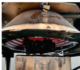
Figure 5. Burning behavior of TPS/10M during cone calorimetry tests.
