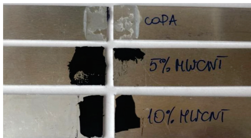
Figure 10. Fracture pattern of joints bonded with MWCNTs modified hot melt at different concentrations.
