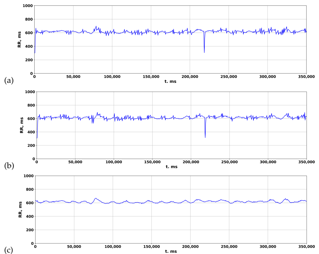
Figure 9. Comparison of rhythmograms in a patient with COVID-19 obtained using different algorithms: (a) Pan–Tompkins; (b) Hamilton; (c) Two-Moving-Average.
