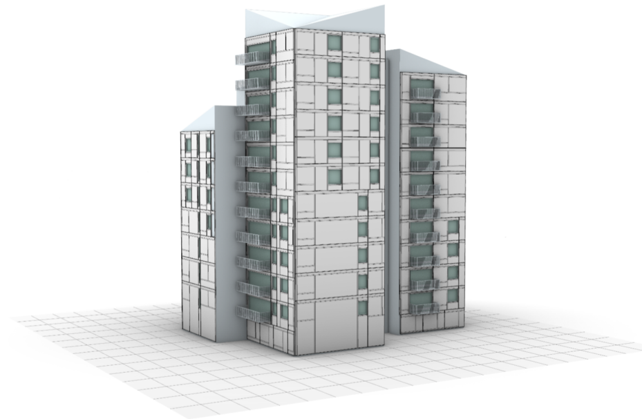
Figure 10. Output of the code described in this section RG1.2, that includes prefabricated layout definition including solar panels and registration areas in the building model of demo-building in Milan, Italy.
