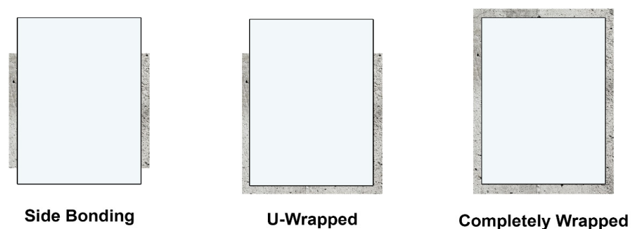
Figure 1. Three wrapping techniques for CFRP in concrete (from left): side, U-wrapping, and complete wrapping.
