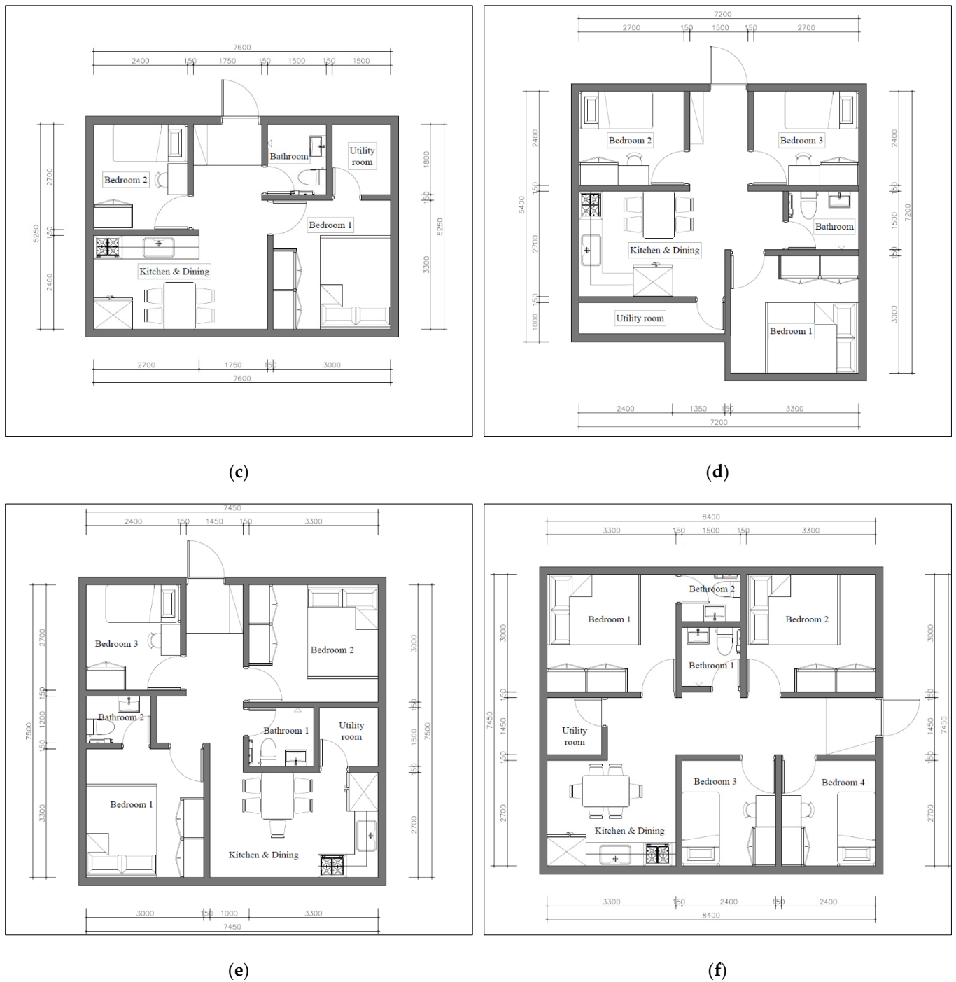
Figure 3. Design simulation of minimum housing standard per household composition (unit: mm): (a) 1-person (18 m 2 ); (b) 2-person (30 m 2 ); (c) 3-person (40 m 2 ); (d) 4-person (48 m 2 ); (e) 5-person (56 m 2 ); (f) 6-person (63 m 2 ).
