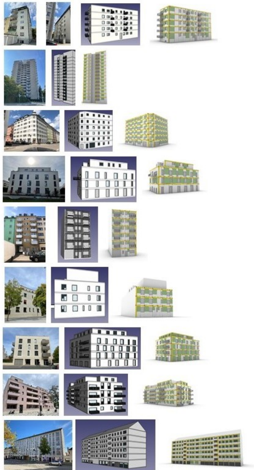
Figure 14. Residential buildings where the tools were applied. In the columns in the left and center, the initial inputs are shown, that is images of the building and the building models. In the column in the right, the building models with the prefabricated module layouts are shown, that is, the output of RG1.2 and RG1.4.
