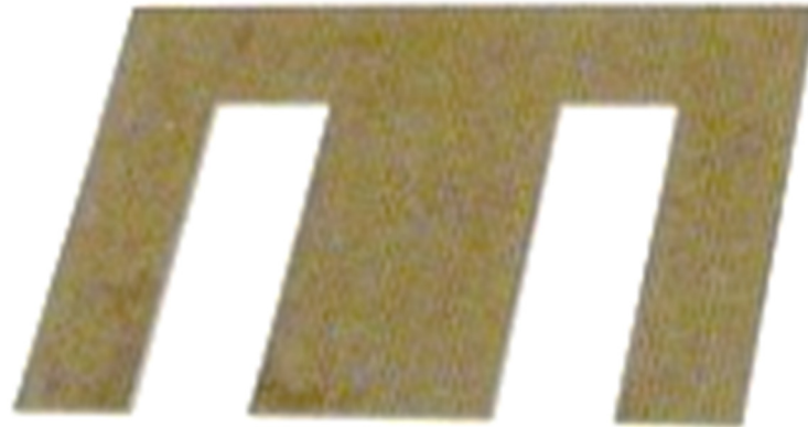
Figure 20. Transformer core sheet cut with optimal technological parameters from grain-oriented electrical steel.
