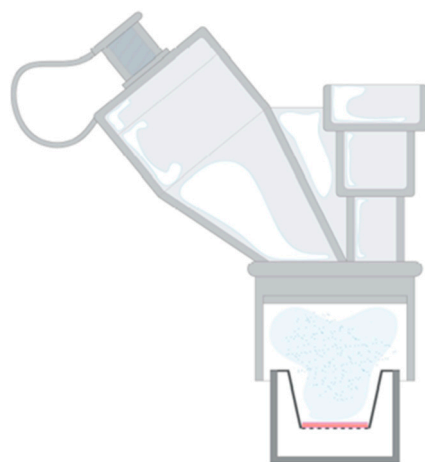
Figure 1. Setup for the direct nebulisation on an ALI monolayer with the Aerogen® Solo™ mesh nebuliser.
