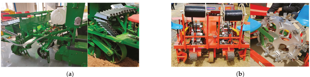
Figure 2. Two kinds of transplanters used for the experiment: (a) finger-clip compound transplanter with its slip transplanting apparatus; (b) clamping-plate compound transplanter with its seedling delivery mechanism.
