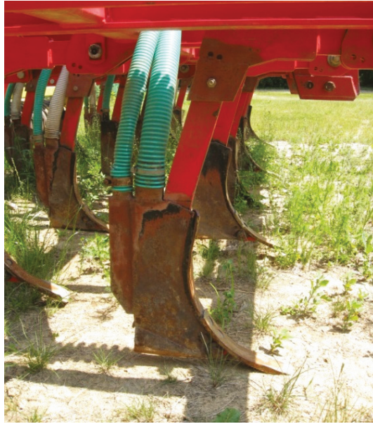
Figure 1. The sweep for deep mineral fertilizer application used in soybean cultivation technology.
