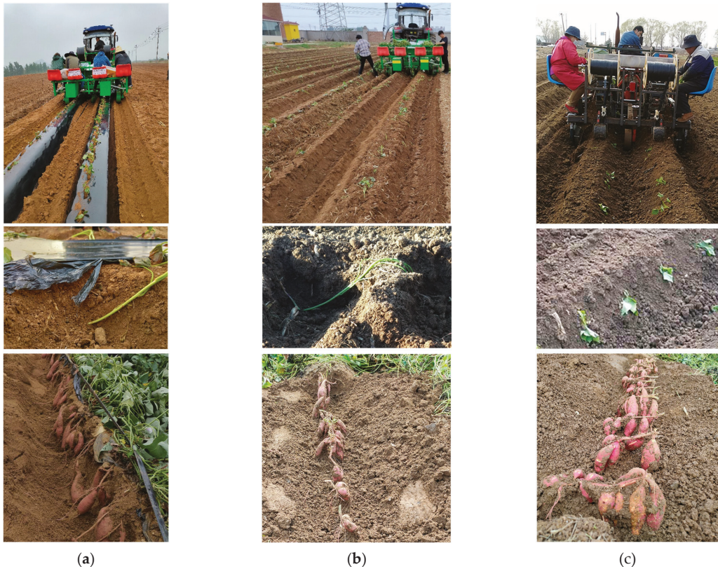
Figure 3. Three designed treatments in this experiment: (a) RB1, finger-clip compound transplanter working under mulched raised beds system; (b) RB2, finger-clip compound transplanter working under bare raised beds system; (c) RB3, clamping-plate compound transplanter working under bare raised beds system.
