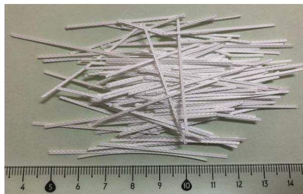
Figure 5. Polypropylene recycled fibres (PPW) with length ranging from 27.1 to 32.6 mm.
