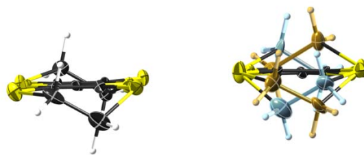
Figure 3. Relative positions in a chain and conformations of terminal ethylene groups for independent BEDT-TTF radical cation A ( left ) and B ( right ) in salt 5. Main positions for disordered ethylene groups of B are colored cyan and complementary are colored navy. The conformation is eclipsed for A and staggered for B. Thermal ellipsoids are of 50% probability.
