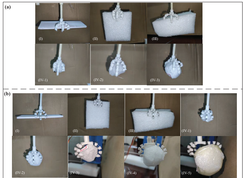
Figure 10. Adaptive performance experiments of two perching grasping mechanisms. (a) Articulated. (b) Elastic reset type. (I) Rectangular cardboard (thin and smooth), (II) rectangular foam object (thicker), (III) irregular foam object (thicker), (IV) near spherical foam object (IV-1)–(IV-5) (diameters approximately 18 mm, 26 mm, 35 mm, 45 mm, 55 mm in that order).
