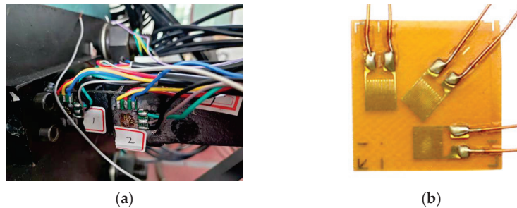
Figure 6. (a) The real configuration of one sensor (strain rosette). (b) The specific structure of one strain rosette.
