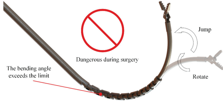
Figure 6. Stability issues of the CTR.
