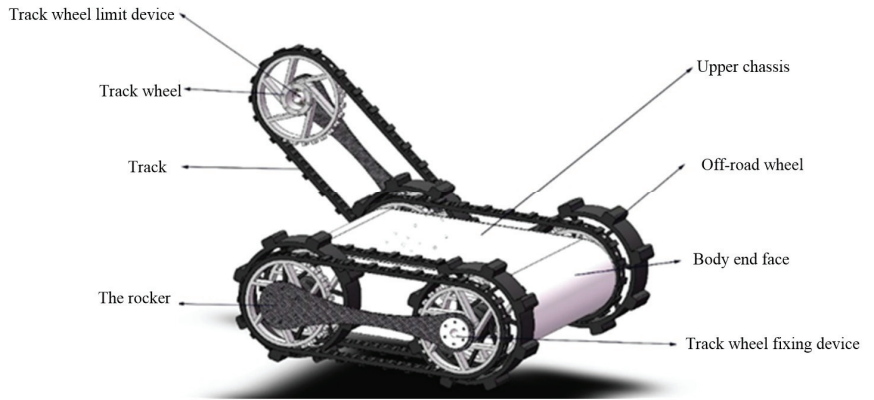
Figure 1. Four-track twin-rocker arm mobile robot object.
