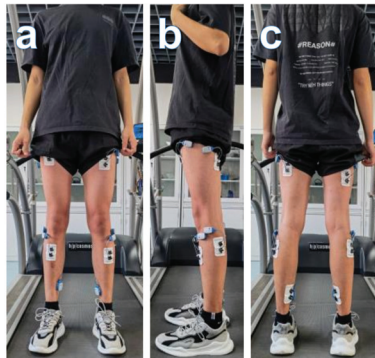
Figure 4. (a) Front, (b) side and (c) rear view of a participant and the placement of electrical electrodes.
