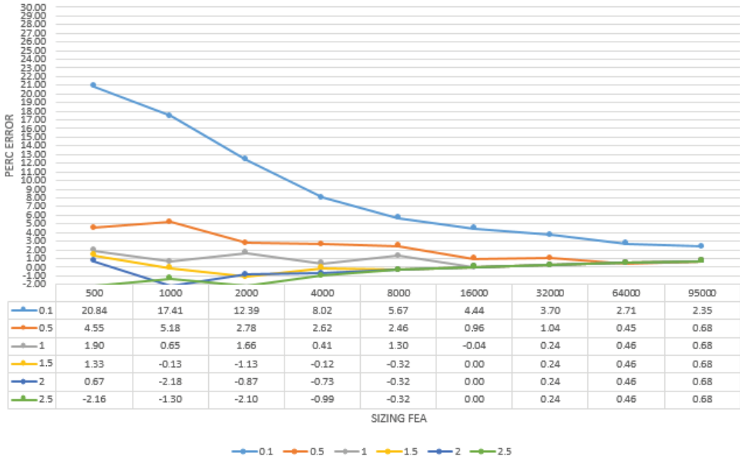
Figure 9. Convergence analysis for the models simplified using retopology with the adaptive size fixed at 30. Highlighted in yellow are the results on convergence expressed in percentage in relation to the result given by the analysis and the analytical result calculated for the specimen. Expressed in a graph.
