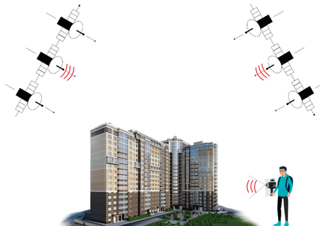
Figure 1. Schematic map of multi-view urban building point cloud acquisition (tomographic synthetic aperture radar system and backpack mobile 3D laser scanner).
