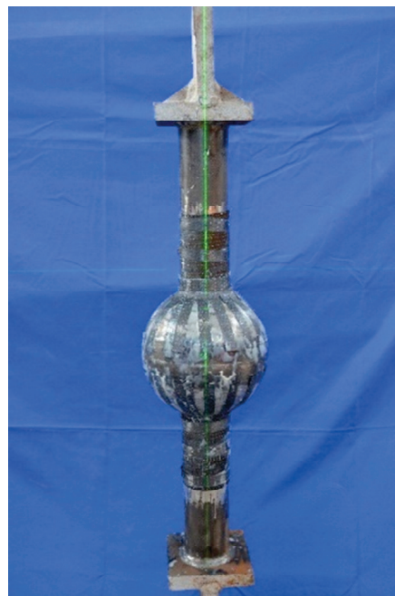
Figure 9. Specimen bonded with CFRP.
