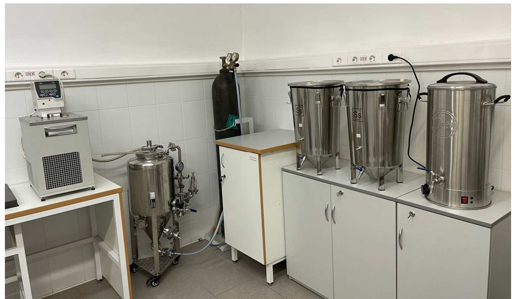
Figure 1. Pilot equipment line for the production of fermented beverages.
