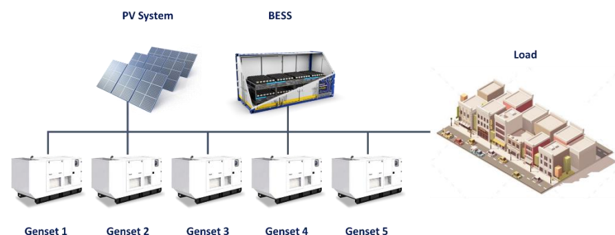
Figure 17. AC Microgrid Topology.
