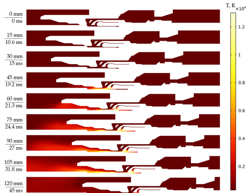
Figure 17. Temperature field (on the left—the contact separation and time).
