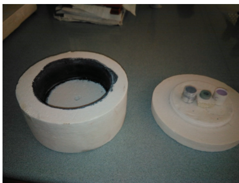
Figure 1. Capsule for microwave kiln painted with SiC.
