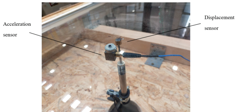
Figure 5. Sensors attached to the sample.
