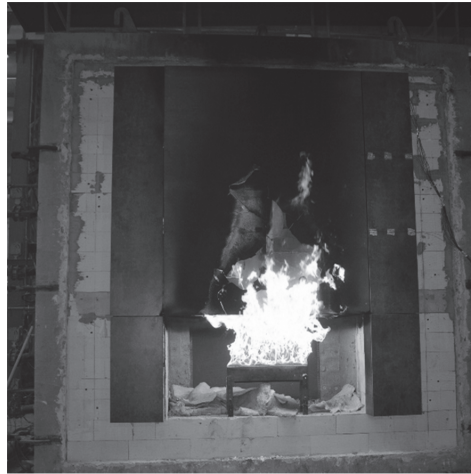
Figure 2. The large scale facade model during exposure to fire.
