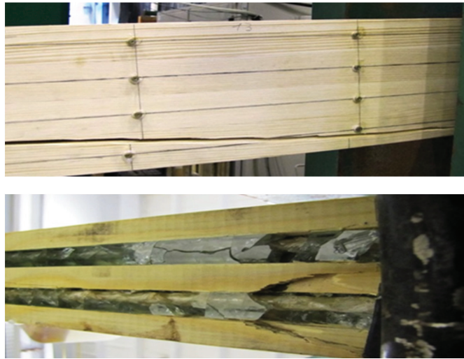
Figure 7. An image of the destruction of the reinforced beams—B3-4.
