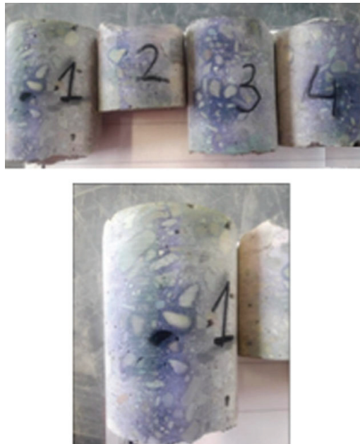
Figure 9. Test of the extension of concrete carbonation.
