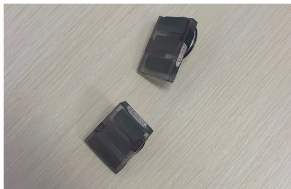
Figure 5. Section samples for scanning microscope examination.
