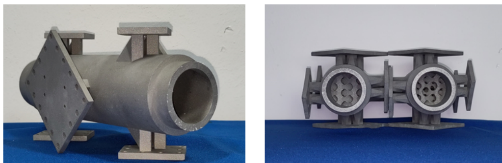
Figure 6. (Left) Manufactured static mixer with connectors for oil channels. (Right) Reference (left) and optimised (right) mixer geometries for validation trials.
