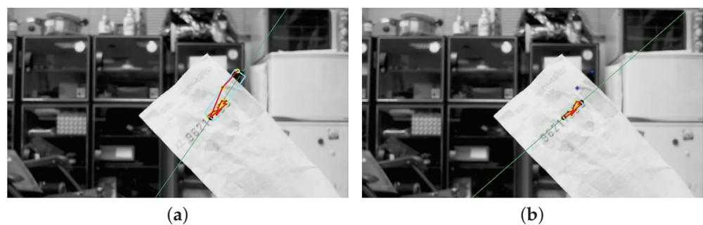
**Figure 8.** Due to the way in which the ordered feature strings are constructed, the outliers commonly appear at the two endpoints. The outlier rejection for the feature points along the text direction based on the distance distribution obtained from OPTICS clustering: (a) OPTICS clustering; (b) with outlier rejection.
