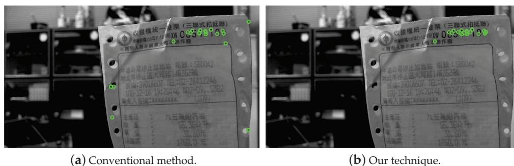
**Figure 3.** The feature extraction results using (a) the conventional method and (b) our technique. The algorithm can reject undesired points while keeping the important features for region detection. It can be seen that our method is able to reject the undesired points while allowing the important features for region detection to remain intact.
