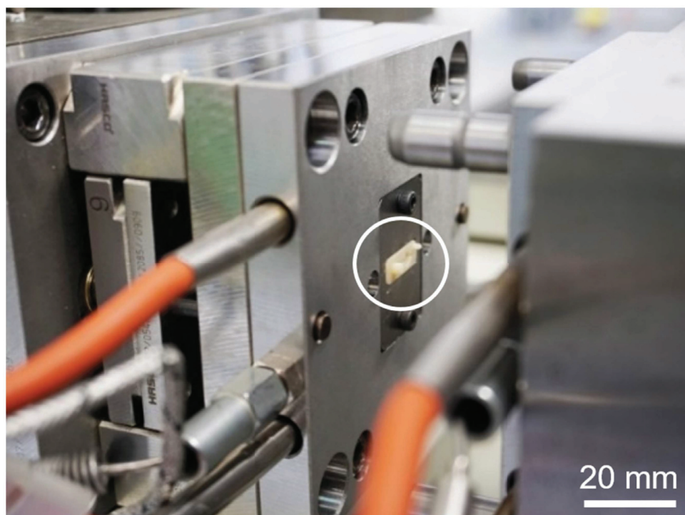
Figure 5. Micro injection molding ( \mu IM) machine equipped with an exemplary 3D-printed mold (see white circle). A metallic holder keeps the mold in position.
