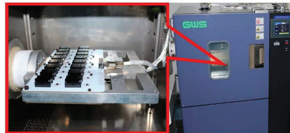
Figure 9. Accelerometer temperature performance test system.
