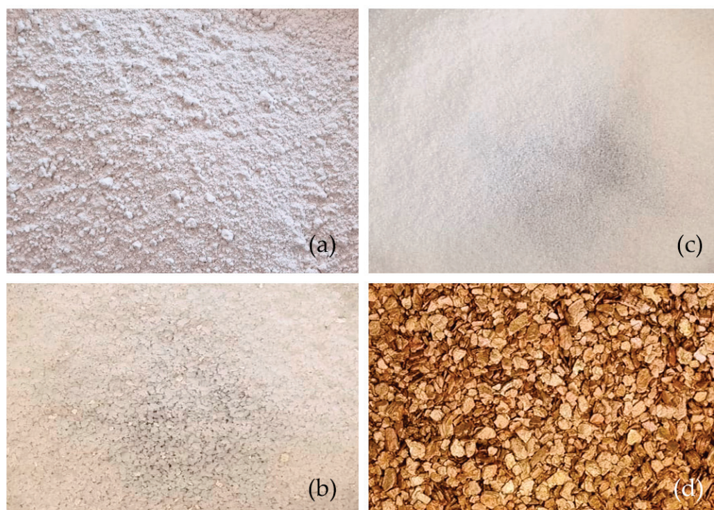
Figure 1. Materials used: (a) gypsum plaster; (b) potassium polyacrylate; (c) sodium polyacrylate; (d) vermiculite.
