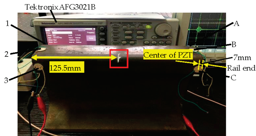
Figure 4. The experimental system for using ultrasonic guided waves detection, in which the position of the red box represents the location of the crack. The PZTs are located at the position of 1, 2, 3, A, B, C, respectively. The distance between the center of PZT and the rail end is 7 mm.
