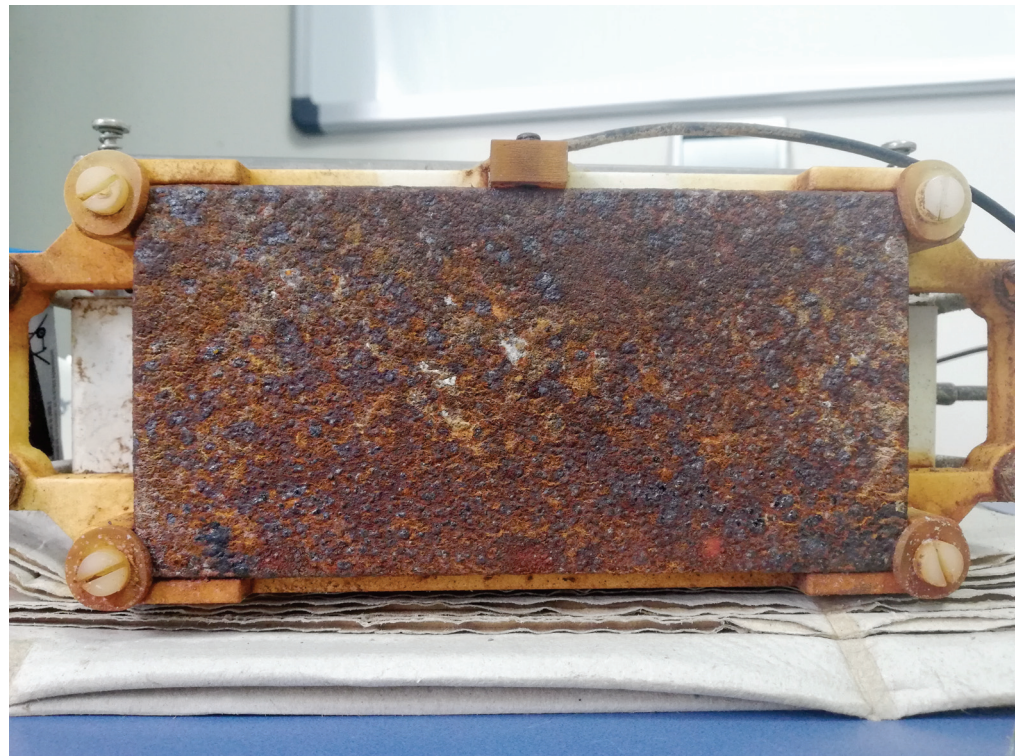
Figure 11. Photo of the bare steel sample after five months of exposure in the Gran Canaria (provided by PLOCAN).
