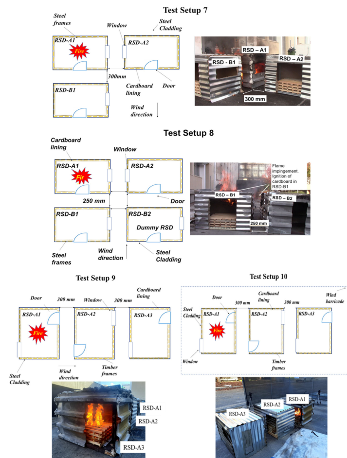
Figure 8. Tests 7 to 10 showing layouts and images during testing.
