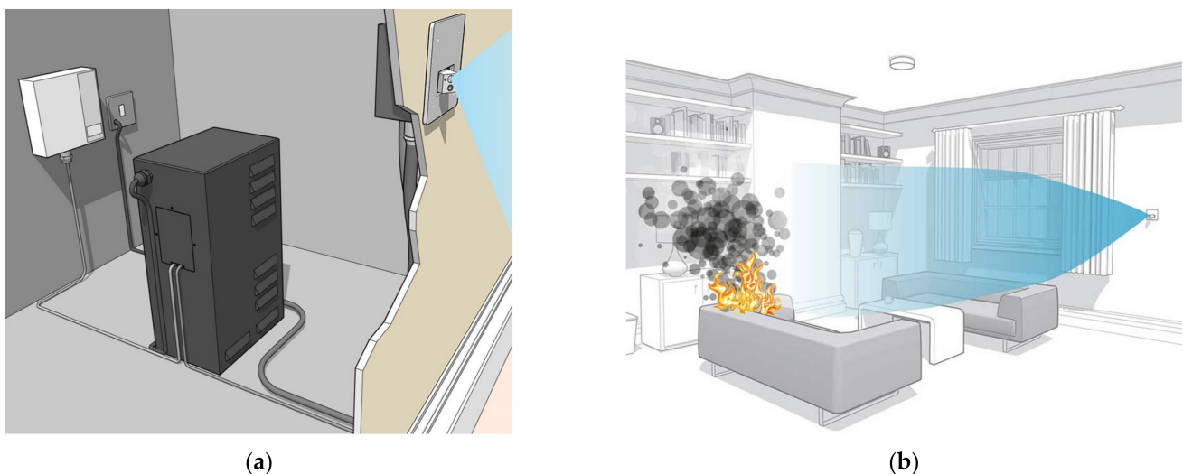
Figure 2. Visualisations of the electronically controlled water mist system: (a) controller and pump; and (b) nozzle discharging water.
