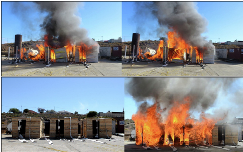
Figure 2. Fire spread between multiple full-scale informal dwellings. (Top) Steel-clad dwellings, (bottom) wooden-clad dwelling [7].
