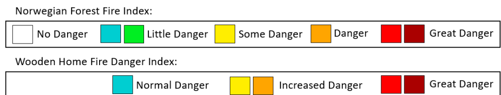
Figure 13. The different levels of danger for the Norwegian Forest Fire Index (Top) and the corresponding suggested levels for the Wooden Home Fire Danger Index (Bottom).
