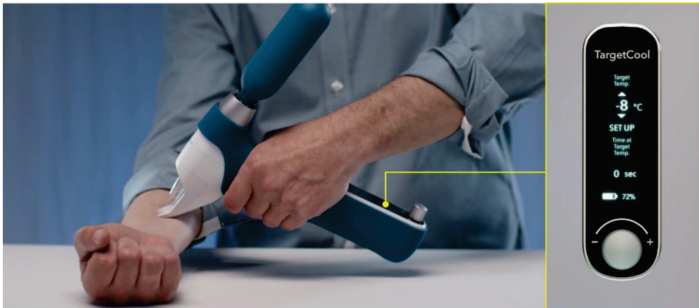
Figure 7. A novel cryotherapy device (TargetCool) developed to provide precise, controlled tissue cooling to reduce pain and inflammation of local procedures. This device uses pressurized carbon dioxide as a cryogen and can actively monitor and maintain the target temperature at a preset temperature (courtesy of RecensMedical, Ulsan, Korea).
