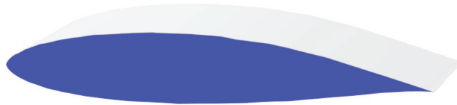
Figure 1. Reference airfoil geometry (NREL S822).
