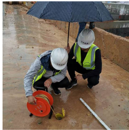
Figure 21. Field picture of groundwater level.
