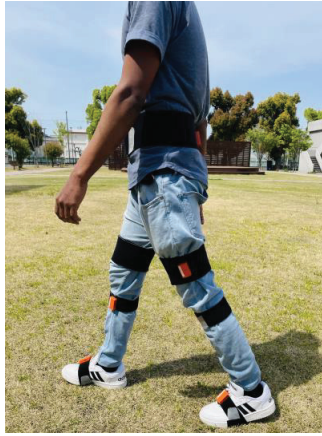
Figure 1. A subject wearing seven Awinda sensors during data acquisition.
