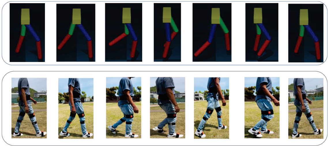
Figure 10. Actual and predicted leg-joint comparison (for the four joint angles) through a graphical simulation.
