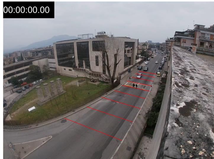
**Figure 9.** Postprocessing video editing to derive speed profiles (red lines represents spaced fixed targets in the video frames every 5 m).
