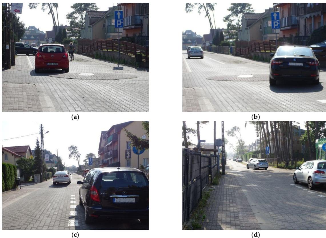
**Figure 16.** Examples of passenger cars driving through traffic circles: (a) traversing the island on the left-hand side; (b) traversing the island on the right-hand side; (c) traversing through the central part of the island; (d) bypassing the island by pulling right. Source: photo by Alicja Sołowczuk.
