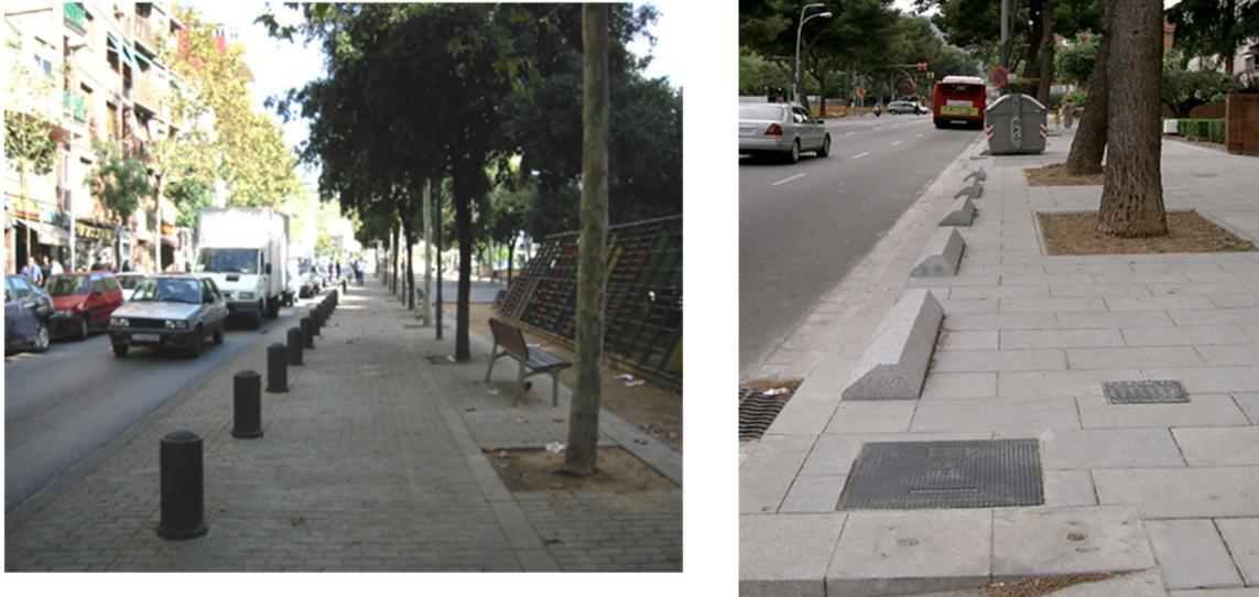
**Figure 11.** Bollards and vegetation restricting the carriageway and/or preventing illegal parking, Barcelona, Spain.
