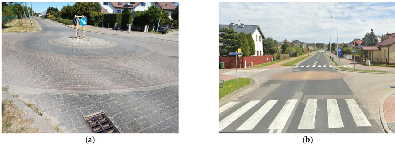
**Figure 3.** Examples of traffic circles used in Poland on two-way streets: (a) an example of a sectioned-off central island on a raised junction in Mierzyn, including traffic signs directing the traffic around the island. Source: photo by Alicja Sołowczuk; (b) example of coloured/textured surface used on the central island of a raised junction in Puławy. Source: Google Earth [5].
