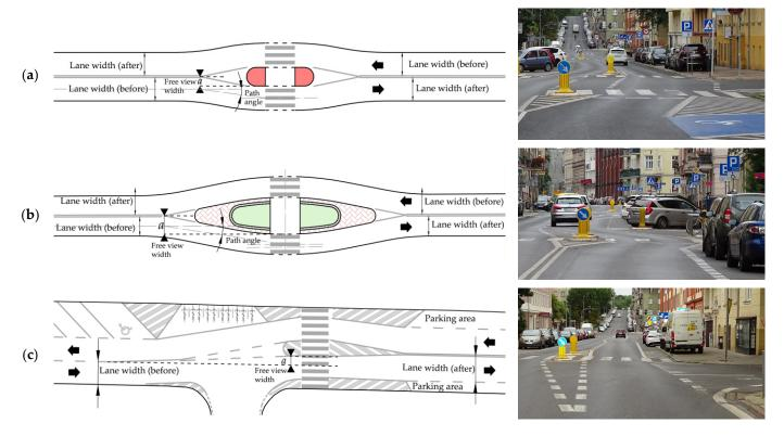
**Figure 1.** Free view and path angle illustration: (**a**) "*a*"—small; (**b**) "*a*"—larger; (**c**) "*a*" +. Source: own work.
