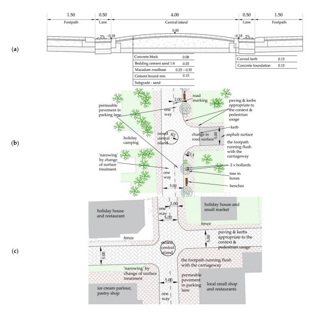
**Figure 10.** Visualization of the analysed traffic circles: (**a**) transverse cross-section; (**b**) plan view of traffic circle No. 2 located on a T-junction; (**c**) plan view of traffic circle No. 7 located on the main promenade (all dimensions in metres). Source: own work.
