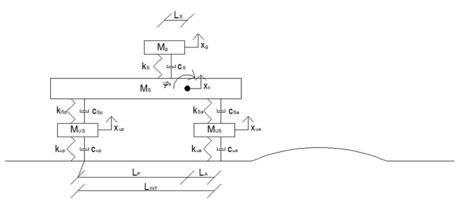
Figure 4. 5 degree-of-freedom (5 dof) vehicle model (half car plus driver insertion).
