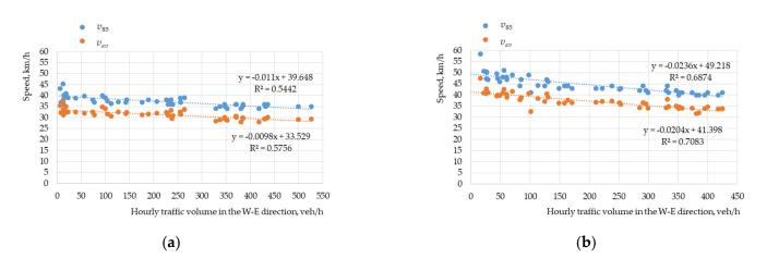
**Figure 9.** Regression analysis examples for different survey station locations: (**a**) at a refuge island; (**b**) on the refuge island approach section. Source: own work.
