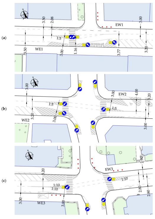
**Figure A1.** Geometrical features of the study sections: (a) WE1 and EW1; (b) WE2 and EW2; (c) WE3 and EW3. (All distances are in metres). Source: own work.
