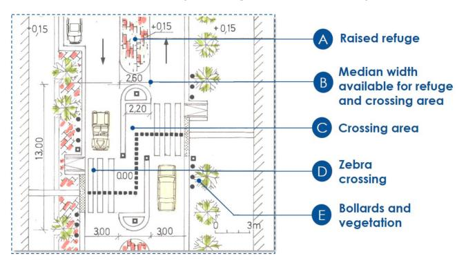
Figure 12. Median opening to create a pedestrian refuge (units in m).
