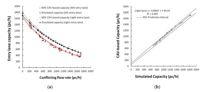
**Figure 4.** The roundabout model built in Aimsun: (**a**) the comparisons between the CAV-based and simulated capacities for the scenario with 60% CAVs and 40% HVDs; (**b**) scattergram analysis for the mixed traffic with 60% CAVs and 40% HDVs (right lane).
