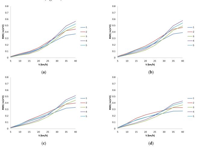
**Figure 5.** (a) Acceleration in terms of RMS on several speed humps (1 to 5) as a function of speed for the vehicle category A; (b) for the vehicle category C; (c) for the vehicle category D; and (d) for the vehicle category E.
