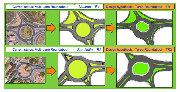
**Figure 3.** Multi-lane existing roundabouts (R1 and R2) and design hypothesis (turbo-roundabouts, TR1 and TR2).
