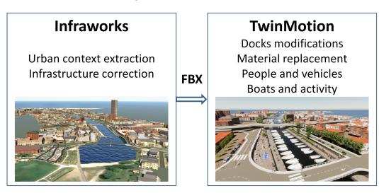
**Figure 3.** Immersive visit design: workflow diagram from GIS urban context extracted with Infra-Works to virtual reality refined scene with TwinMotion.
