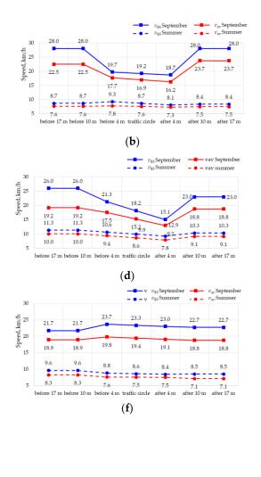
**Figure 17.** Traffic circle driving speed profiles: (a) No.  $1-\Delta h = 0.12$  m; (b) No.  $2-\Delta h = 0.09$  m; (c) No.  $3-\Delta h = 0.17$  m; (d) No.  $4-\Delta h = 0.16$  m; (e) No.  $5-\Delta h = 0.12$  m; (f) No.  $6-\Delta h = 0.08$  m; (g) No.  $7-\Delta h = 0.11$  m. Source: own work.
