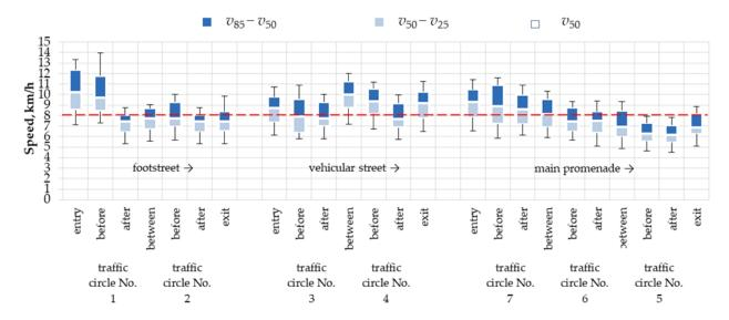
**Figure 12.** Box plot of speed data measured in summer. The whiskers represent the minimum and maximum values; lower and upper edges of the boxes determine the first and third quartiles; the bold white line designates the median value (the arrow indicates the direction of movement). Source: own work.
