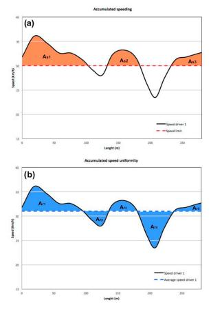
**Figure 2.** Example of evaluation of the areas for the definition of the effectiveness indicators: (a) accumulated speeding; (b) accumulated speed uniformity.
