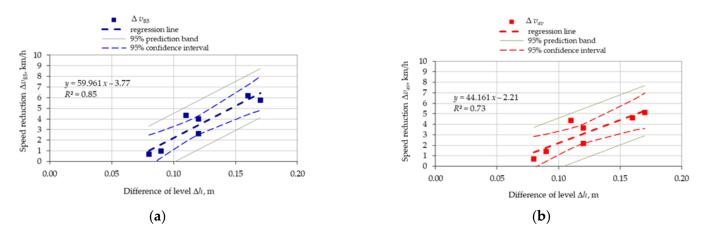
**Figure 18.** Speed reduction vs. central island difference of level  $\Delta h$ : (a)  $v_{85}$ ; (b)  $v_{av}$ . Source: own work.
