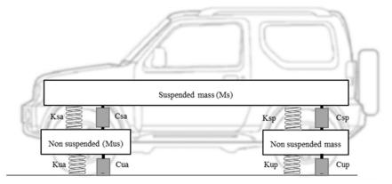
Figure 3. 4 degree-of-freedom (4 dof) vehicle model (half car).
