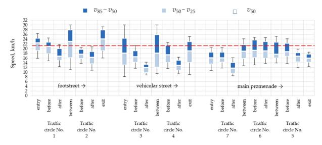
**Figure 13.** Box plot of speed data measured in September. The whiskers represent the minimum and maximum values; lower and upper edges of the boxes determine the first and third quartiles; the bold white line designates the median value (the arrow indicates the direction of movement). Source: own work.
