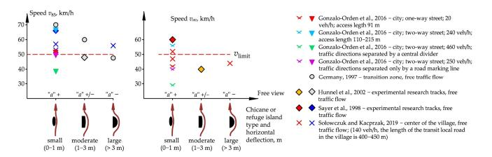
**Figure 2.** Comparison of  $v_{85}$  and  $v_{av}$  values ahead of a refuge island or median island in different locations. Source: Own work based on data presented in: Gonzalo-Orden et al., 2016 [28], Germany, 1997 [39], Hunnel et al., 2002 [40], Sayer et al., 1998 [37], Sołowczuk & Kacprzak, 2019 [21].
