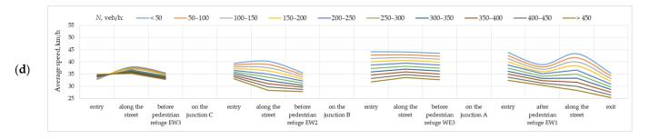
**Figure 10.** Speed distribution along the analysed street: (**a**) 85th percentile speed in the direction  $W \rightarrow E$ ; (**b**) average speed in the direction  $W \rightarrow E$ ; (**c**) 85th percentile in the direction  $E \rightarrow W$ ; (**d**) average speed in the direction  $E \rightarrow W$ . Source: own work.
