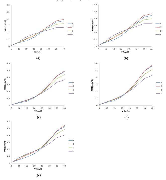
**Figure 6.** (a) Acceleration in terms of RMS on different classes of vehicles (A to E) caused by the speed hump 1; (b) by the speed hump 2; (c) by the speed hump 3; (d) by the speed hump 4; and (e) by the speed hump 5.
