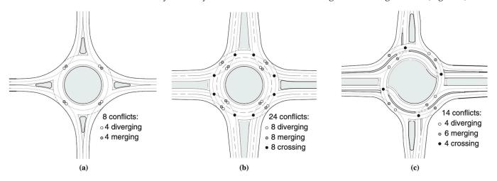
Figure 1. Conflict points (a) single-lane roundabout; (b) double-lane roundabout; (c) turbo-roundabout.
