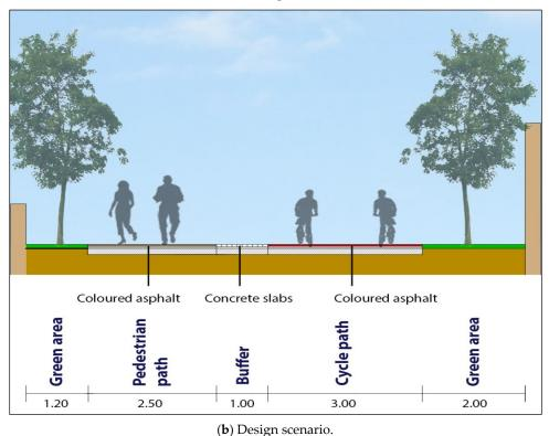
Figure 10. Pedestrian and bicycle routes in the layout of roads for motorized vehicles: existing (a) and
