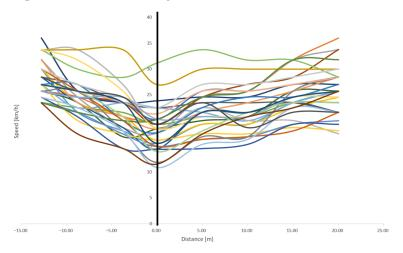
**Figure 10.** Speed profiles, represented in several colors in the graph, of a typical working daytime slot in the forward direction "a". Zero distance identifies the RPC location.
