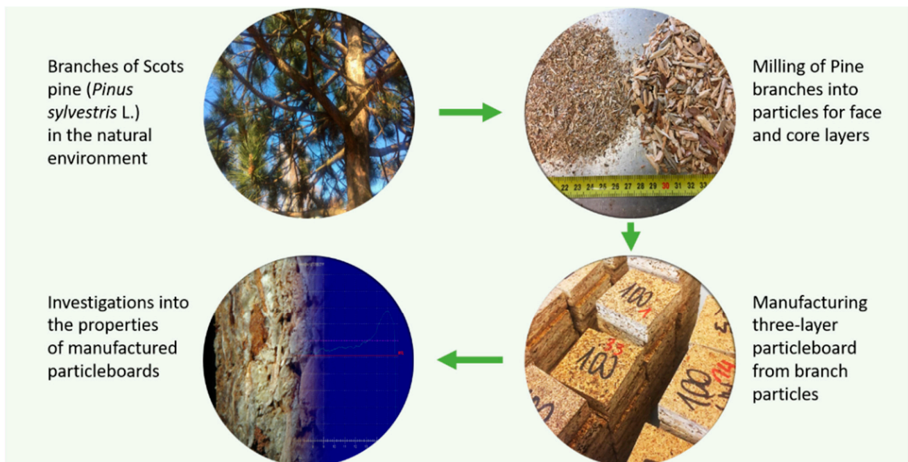
Figure 2. The general production process of three-layer particleboard from pine branches.
