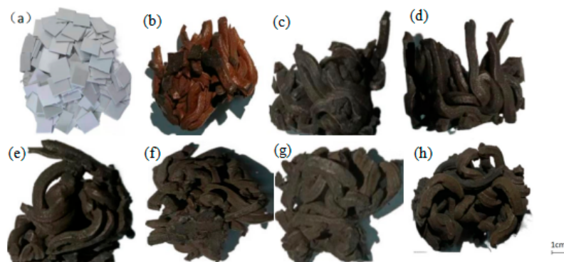
Figure 2. Morphology of PVC film heated at different temperatures: (a) PVC film pieces, (b) 280 \text{°C} , (c) 310 \text{°C} , (d) 340 \text{°C} , (e) 370 \text{°C} , (f) 400 \text{°C} , (g) 430 \text{°C} , (h) 460 \text{°C} .
