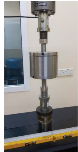
Figure 7. Product testing, showing force–displacement test and results for product under cyclical compression.
