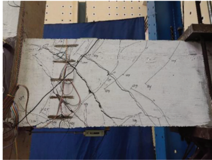
Figure 10. Test phenomenon of specimen J-2.
