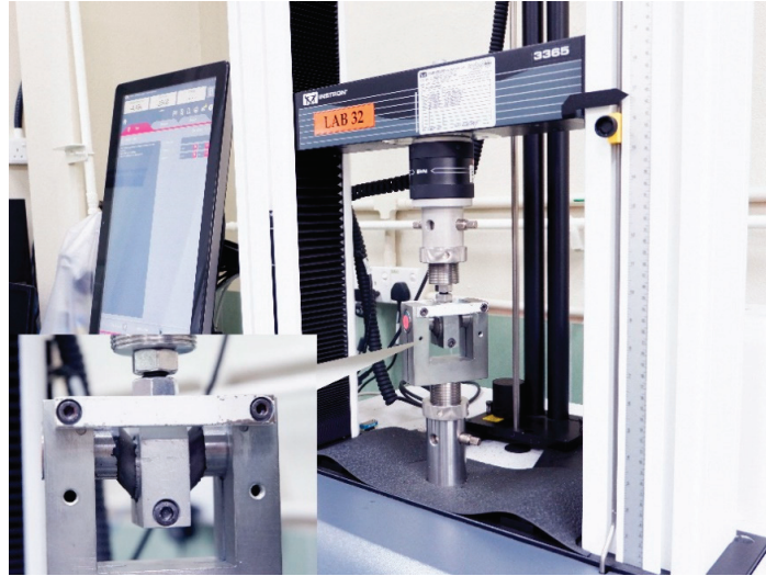
Figure 2. Double-shear testing using INSTRON servo-hydraulic testing machine.
