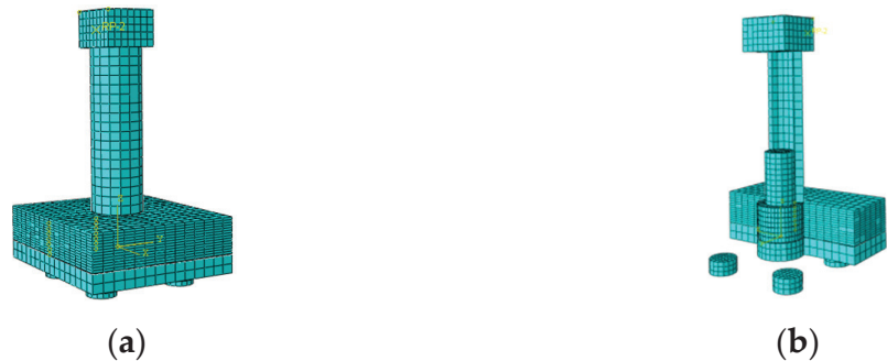
Figure 12. Finite element model of the improved socket connection. (a) Precast member; (b) sectional view of the model.
