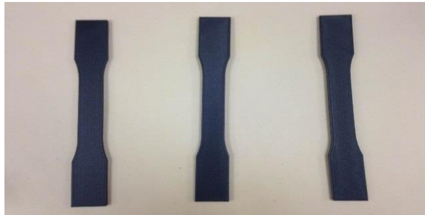
Figure 1. ASTM D 638 Tensile Specimens (6 inches long).
