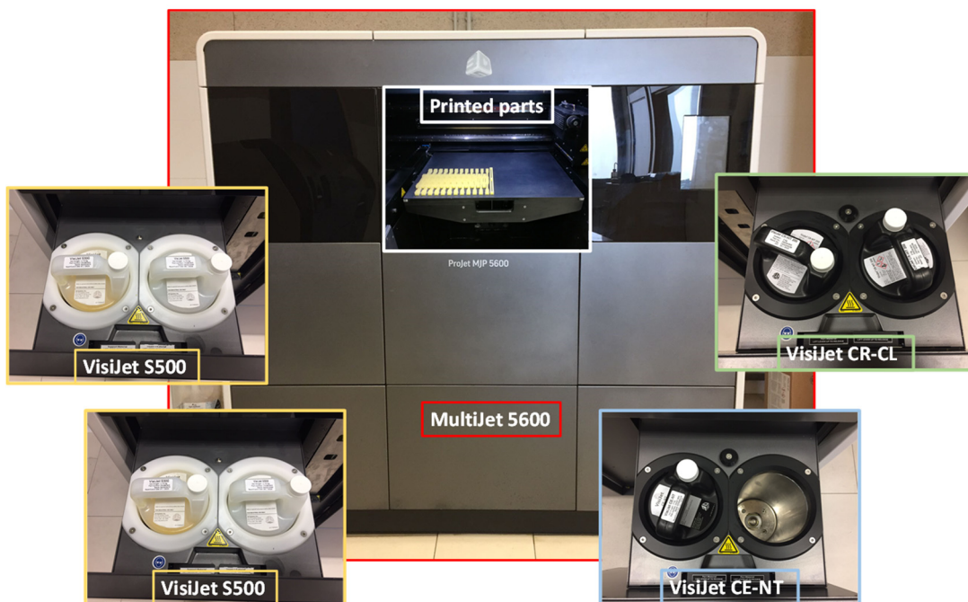
Figure 2. Project MJP 5600 machine with a set of specimens and VisiJet materials.
