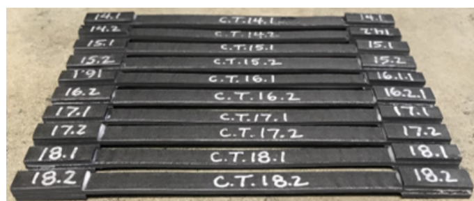
Figure 3. Photo of 13% CF-ABS tensile specimens prior to testing.
