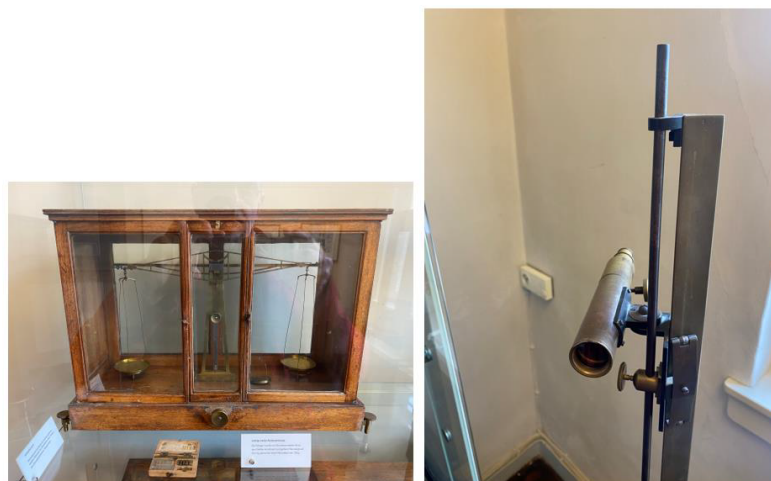
Figure 12. The best balance of Liebig with an accuracy of 0.3 mg and a maximum of 100 g; the telescope used to read the balance.
