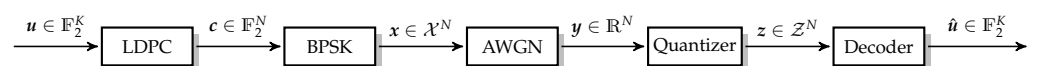
Figure 1. Transmission model for transmission of LDPC encoded messages over an AWGN channel with quantization prior to FEC decoding.
