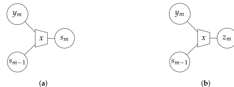
Figure 11. Graphical illustration of IB fusion of two inputs to determine instantaneous side-information s_m (a) and the quantizer sensor output z_m (b) for a successive point-to-point transmission of instantaneous side-information.
